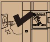
**4. If you want to clean the machine or you don't run the machine for a long time, please unplug the power cord and loose the draining nut to drain off the water.**
